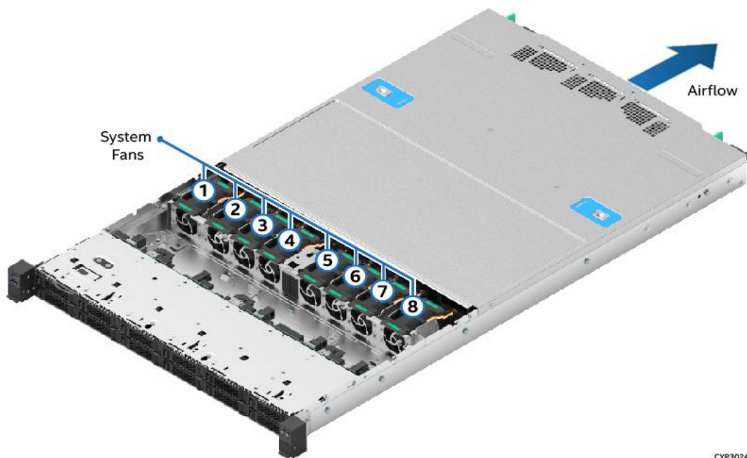
Figure 36. System Airflow and Fan Identification
