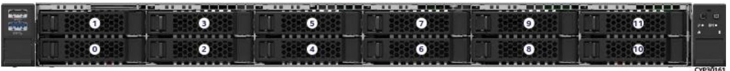
Figure 58. 12 x 2.5" Front Drive Bay Configuration – M50CYP1UR212
