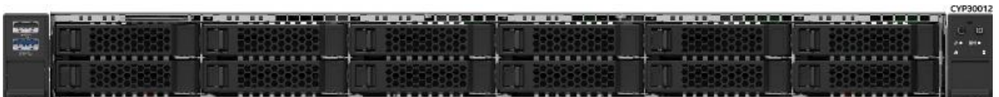
Figure 6. 12 x 2.5" Front Drive Bay Configuration – M50CYP1UR212
