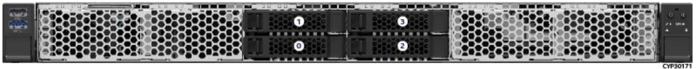
Figure 57. 4 x 2.5" Front Drive Bay Configuration – M50CYP1UR204
