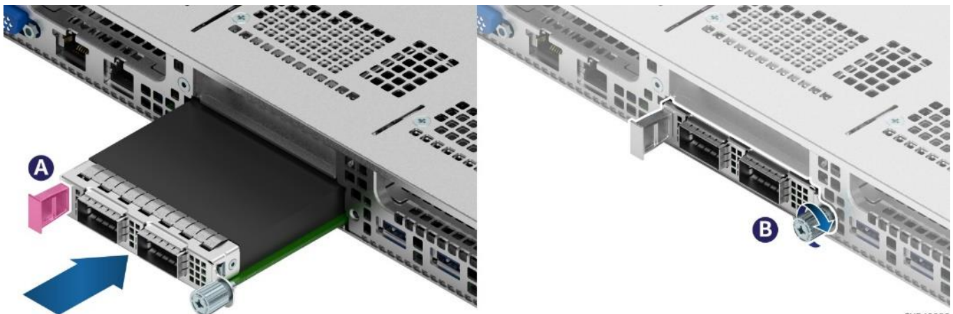
Figure 56. OCP* Adapter with Pull Tab Installation
