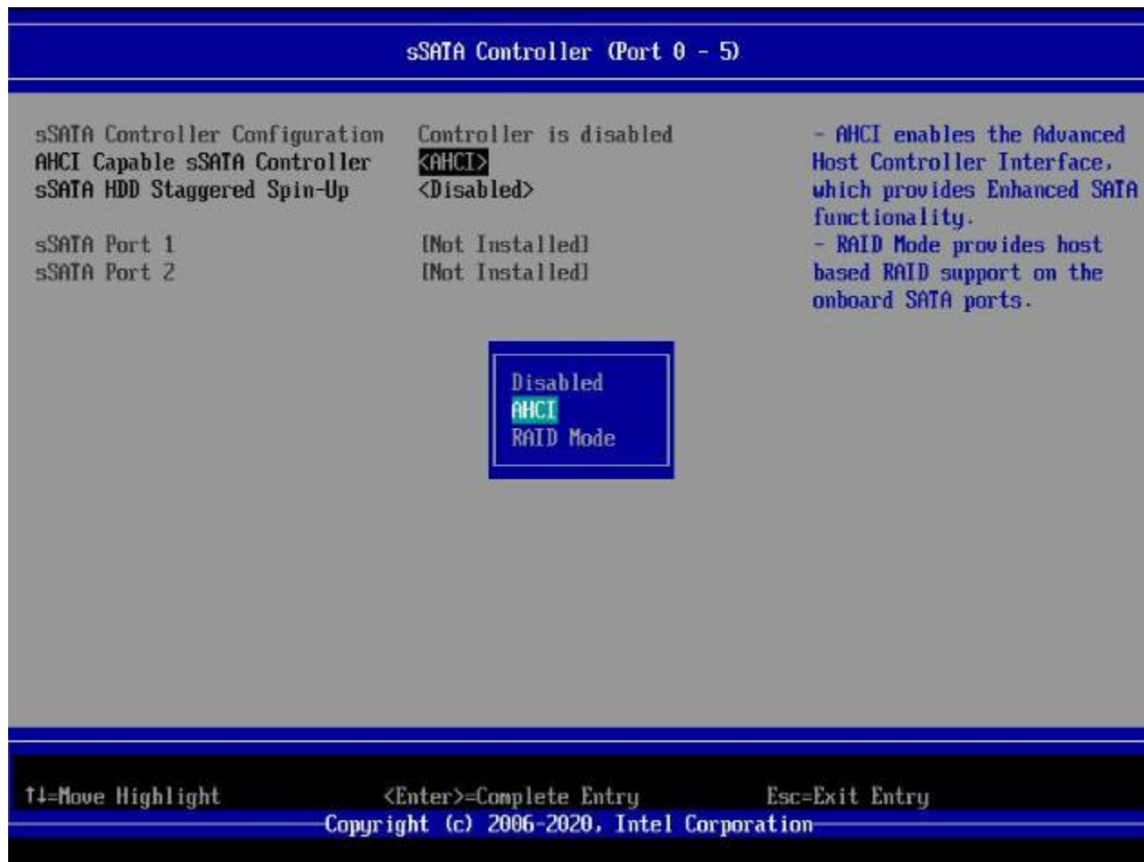
Figure 86. BIOS Setup Mass storage Controller Configuration Screen
