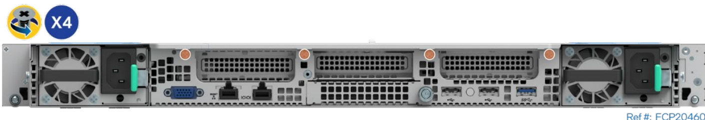
Figure 90. Chassis Riser Card Bracket Screws
