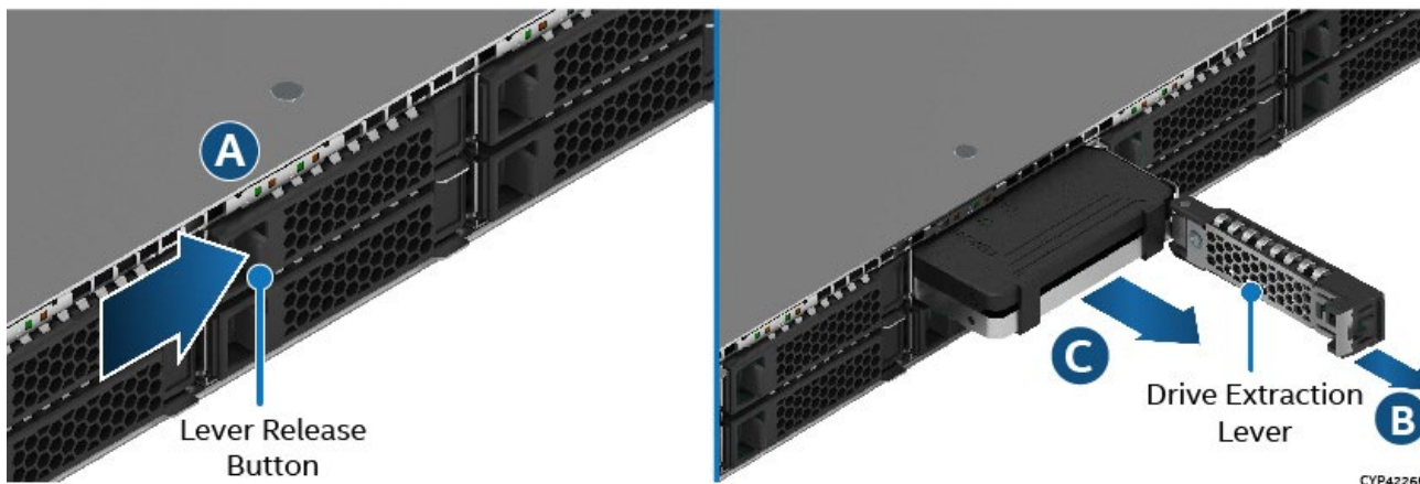
Figure 38. Drive Blank Removal
