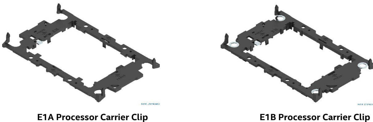
Figure 9. Supported Processor Carrier Clips
