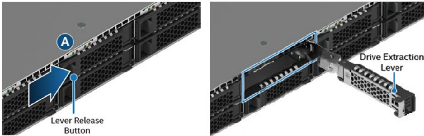
Figure 102. Drive Extraction Lever Release
