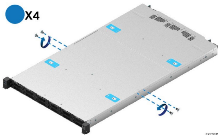
Figure 65. System Top Cover Panel Shipping Screws
