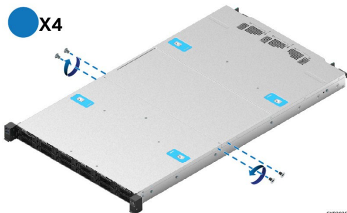
Figure 24. System Top Cover Panel Shipping Screws
