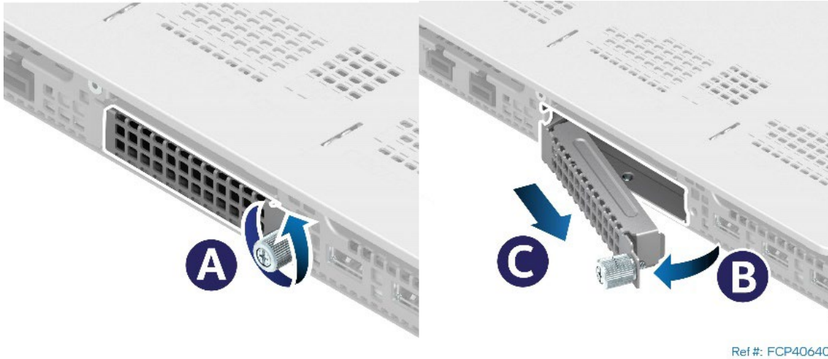
Figure 43. OCP* Adapter Bay Filler Removal
