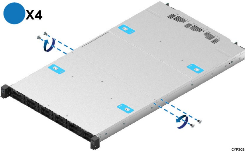
Figure 4. System Top Cover Panel Shipping Screws
