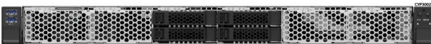
Figure 54. 4 x 2.5" Front Drive Bay Configuration–M50FCP1UR204
